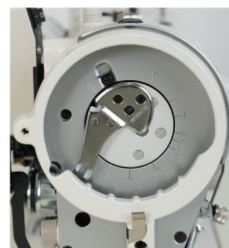
旋轉式挑線桿/ Rotary Thread Take-up Lever
