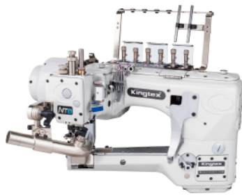
NTD7701 4-Needle, 6-Thread Flat-Seamer, Feed-Off-The-Arm Machine
