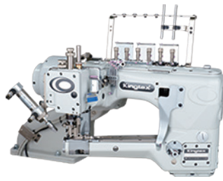
NTD77 / TC026 FEED-OFF-THE-ARM MACHINE FOR FLAT SEAMING
