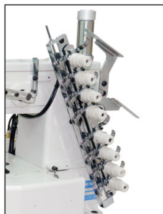
UT04A 鬆線組 Thread tension release
