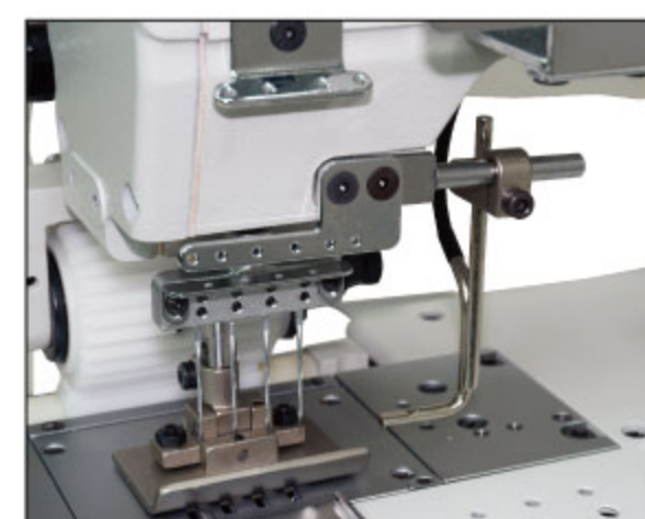
撥線裝置 Thread tension releaser
