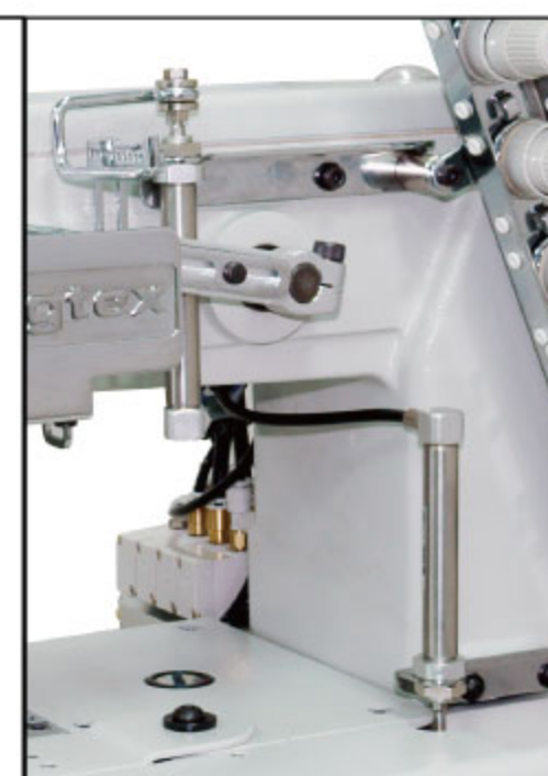
UT12A 鬆線組 Thread tension release
