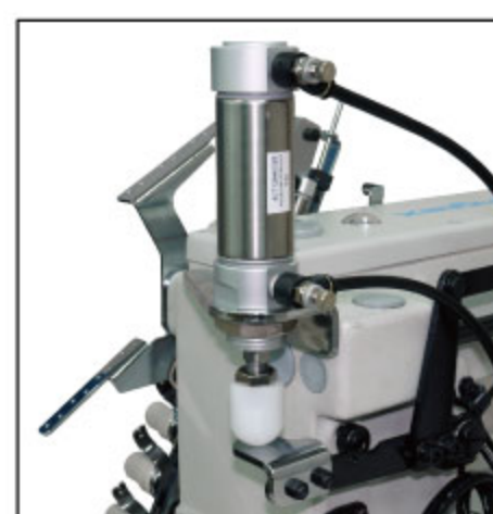
AL004:自動抬壓腳 Presser foot lifter
